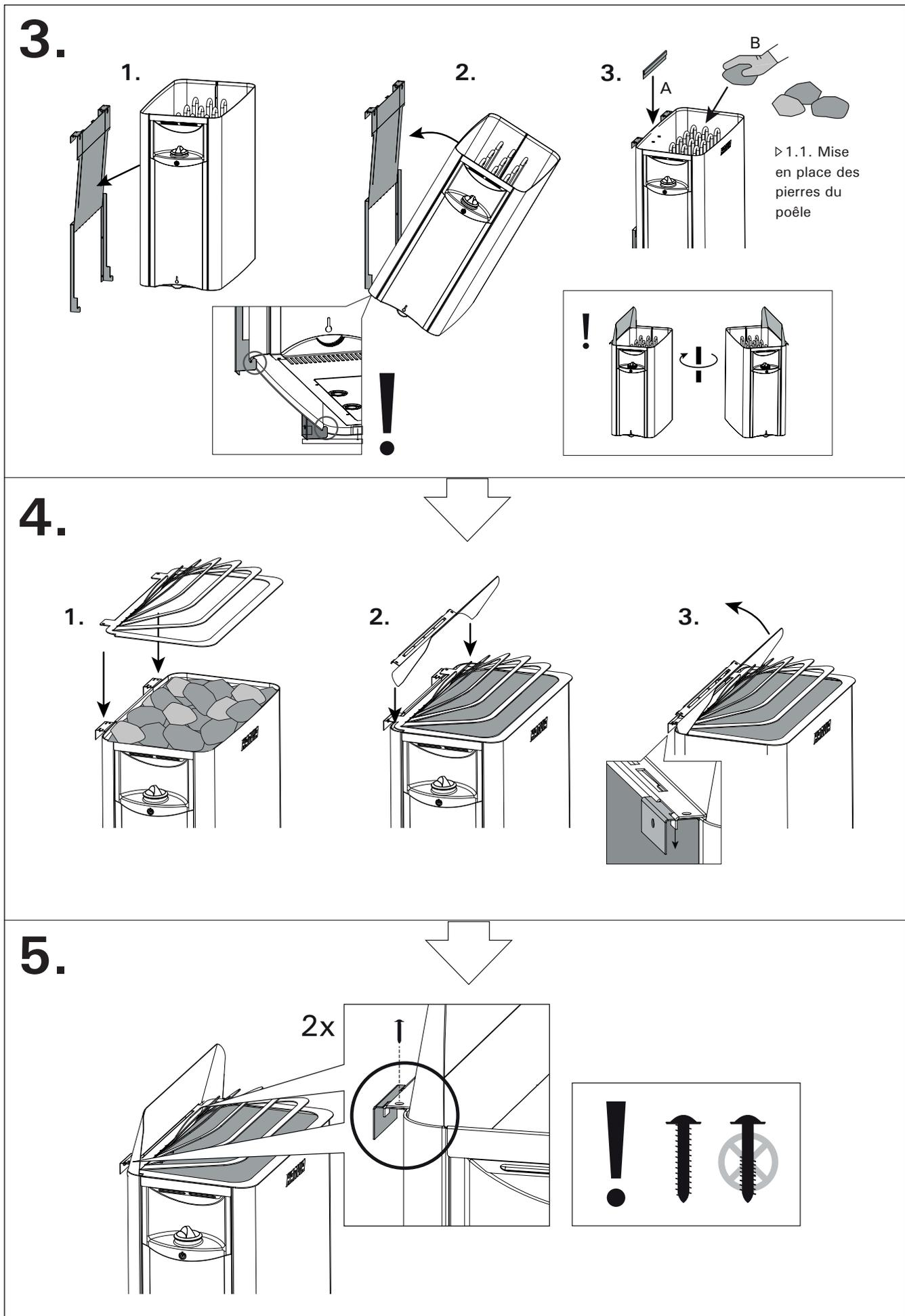
Figure 7. Installation du support mural. (2.) and the heater (3.-5.).
