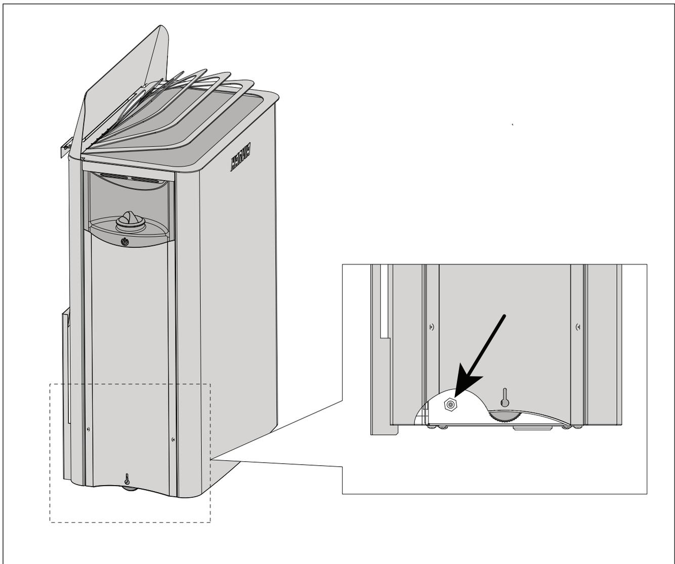
Figure 8. Reset button for overheat protector.
