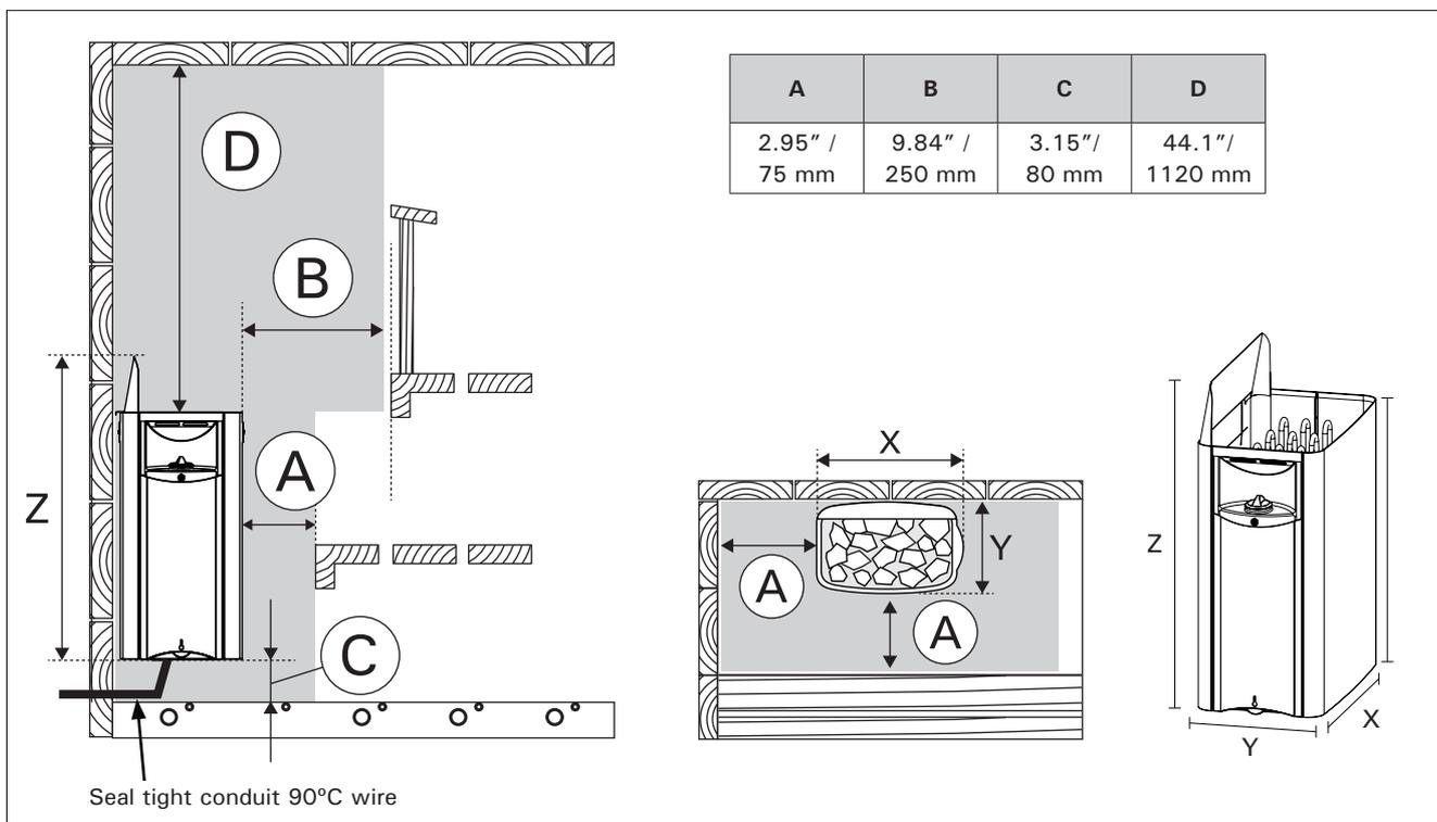
Figure 4. Minimum safety distances (all heater models).
