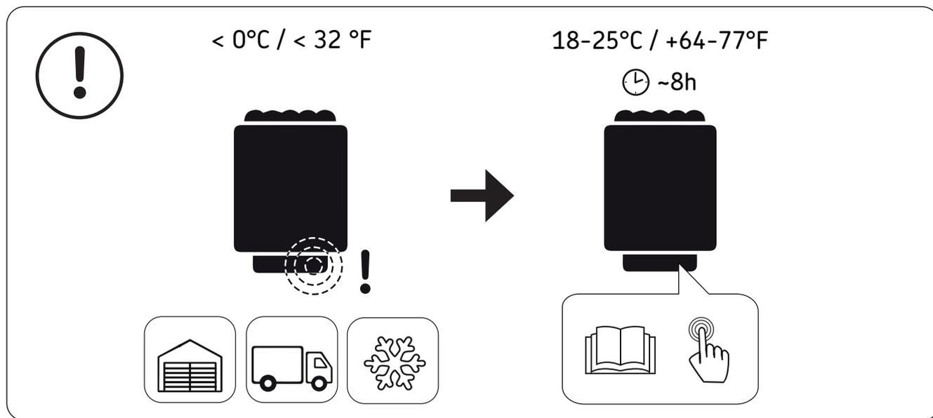
**EN:** Overheat protector of the device can go off also at temperatures below  $-5^{\circ}\text{C}$  /  $23^{\circ}\text{F}$  (storage, transport, environment). Before installation take the device to the warm environment. The overheat protector can be reset when the temperature of the device is approx  $18^{\circ}\text{C}$  /  $64^{\circ}\text{F}$ . **The overheat protector must be reset before using the device.** See the user manual > Resetting the Overheat Protector.
