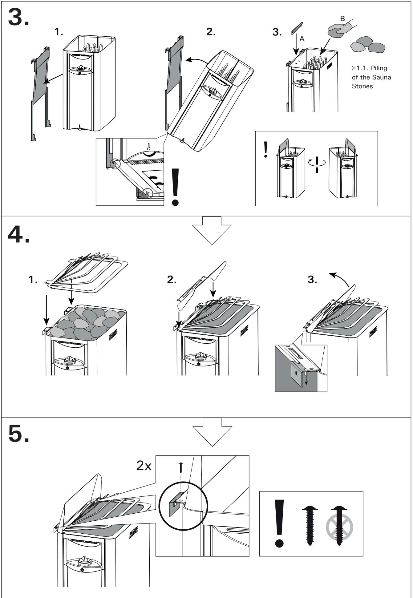
Figure 7. Installing the wall-mounting device (2.) and the heater (3.-5.)
